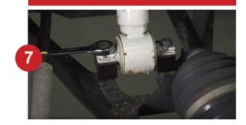
Insert the bolts from the top down so that the nut is on the bottom. If the bolts come from the bottom they will contact the CV. shaft.
