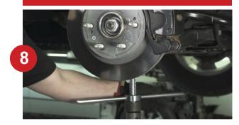
Raise the lower control arm to raise the spindle while lowering the upper control arm to re-install the upper ball joint and Re-install the steering linkage.
