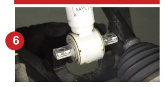
You can then insert the spacer between the lower control arm and the lower strut mount and align the holes.
