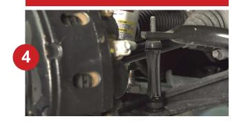
Remove the sway bar nut and bushing.
