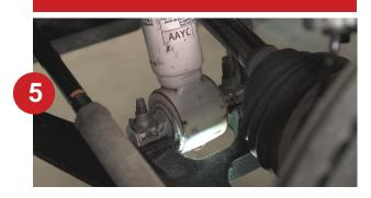
Remove the two lower strut mount bolts and loosen the 3 upper strut mount nuts. Remove the two lower spring clip nuts and discard.
