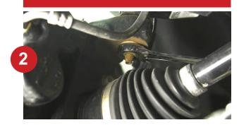
Use an 18mm wrench to remove the upper strut mount nuts and the upper ball joint nut. Strike the side of knuckle with a hammer to get the ball joint to separate.
