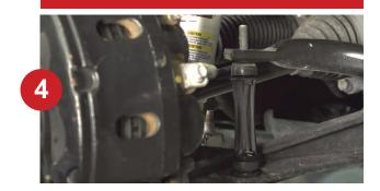
Remove the sway bar nut and bushing.
