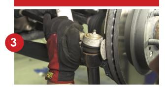
Using a 21mm wrench, remove the steering linkage nut.
