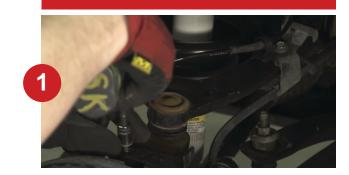
After removing the wheel, remove any brake line and ABS line brackets, so you have enough slack in the lines.
