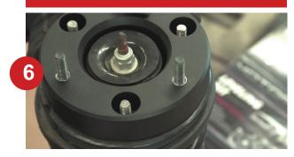
Install the supplied bolts into the leveling kit spacer. These will act as the new studs when reinstalled. Bolt the spacer to the top of the strut using the supplied nuts.
