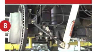
Complete the installation on the other side of the truck before reinstalling any brake or ABS lines. After 100 miles recheck torque to factory spec.
