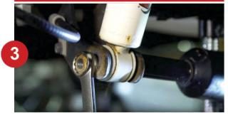
Remove the lower rear shock mount nut and bolt.
