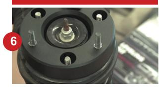
Install the supplied bolts into the leveling kit spacer. These will act as the new studs when reinstalled. Bolt the spacer to the top of the strut using the supplied nuts.
