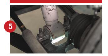
Remove the two lower strut mount bolts and remove the strut from the vehicle.
