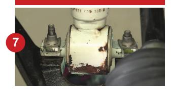
Rotate the strut 180 degrees and install it back into the truck. Re-insert the lower strut bolts.
