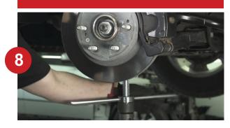
Raise the lower control arm to raise the spindle while lowering the upper control arm to re-install the upper ball joint and Re-install the steering linkage.
