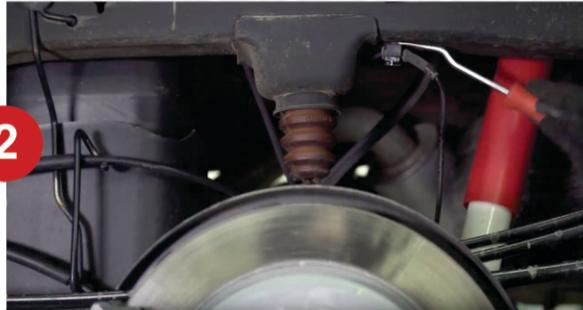
2 Remove the brake and parking brake cables so there is slack in the lines.
