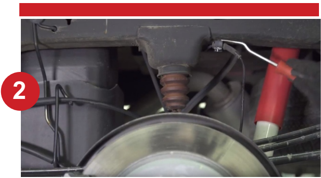
Remove the brake and parking brake cables so there is slack in the lines.
