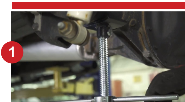
Support the rear axle with a jack and jack stands.
