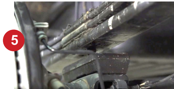
5 Lower the axle so you can install the new rear block.
