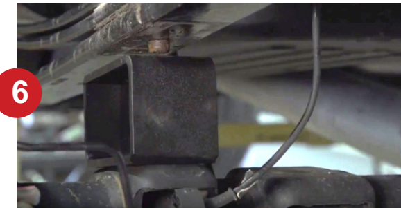
6 Install the new rear block making sure the smaller side of the spacer is facing the front of the truck
