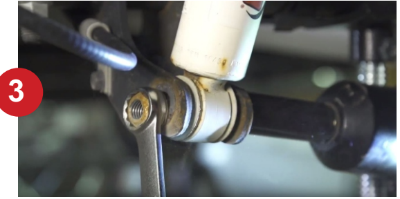
3 Remove the lower rear shock mount nut and bolt.
