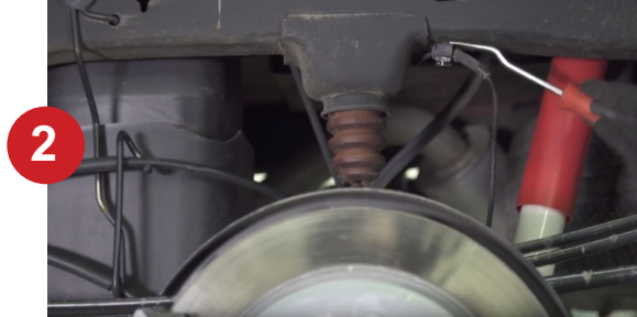
2 Remove the brake and parking brake cables so there is slack in the lines.
