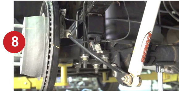
8 Complete the installation on the other side of the truck before reinstalling any brake or ABS lines. After 100 miles recheck torque to factory spec.
